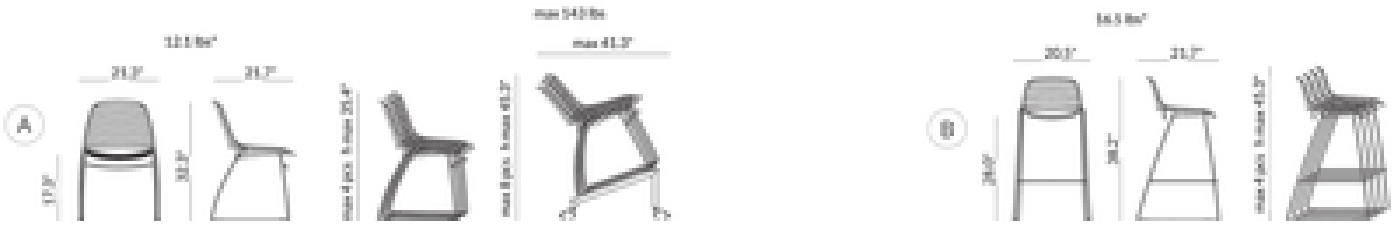
Eclipse Wire: A chair, B stool. Technical drawing reproduced from the 2026 Listino Urbantime. Dimensions are in inches; weights in pounds.
